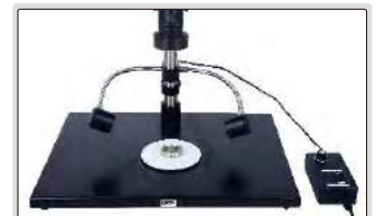
illumination direction and brightness are adjustable
