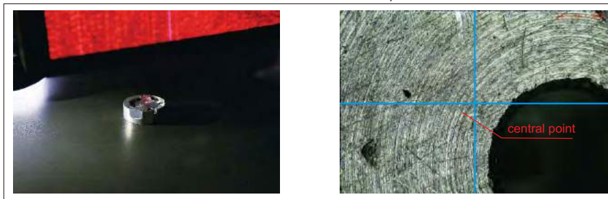
laser indicator locates the central point
