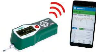
operate roughness tester by mobile phones
