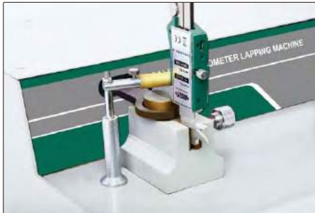
lapping measuring surfaces of caliper lower jaws
