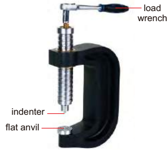
static test clamp
