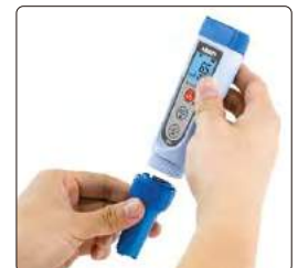
electrodes can be replaced
