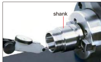
measure radial runout of shank
