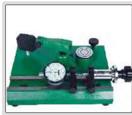
inspect accuracy of dial indicators (range 0-25mm)
