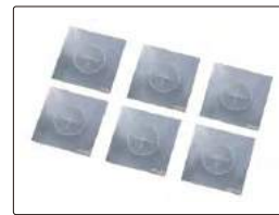
A1 standard sensitivity test piece (optional)
