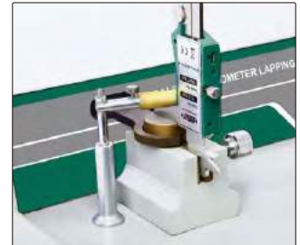
lapping measuring surfaces of caliper lower jaws
