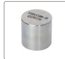
15# carbon steel control sample (optional)
