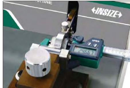
lapping measuring surfaces of outside micrometer
