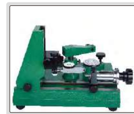
inspect accuracy of test indicators
