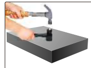
hammer impact to apply test force
