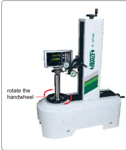
rotate the handwheel to rotate tools
