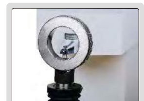
measure interior of pipes and grooves, the minimum internal diameter is 35mm
